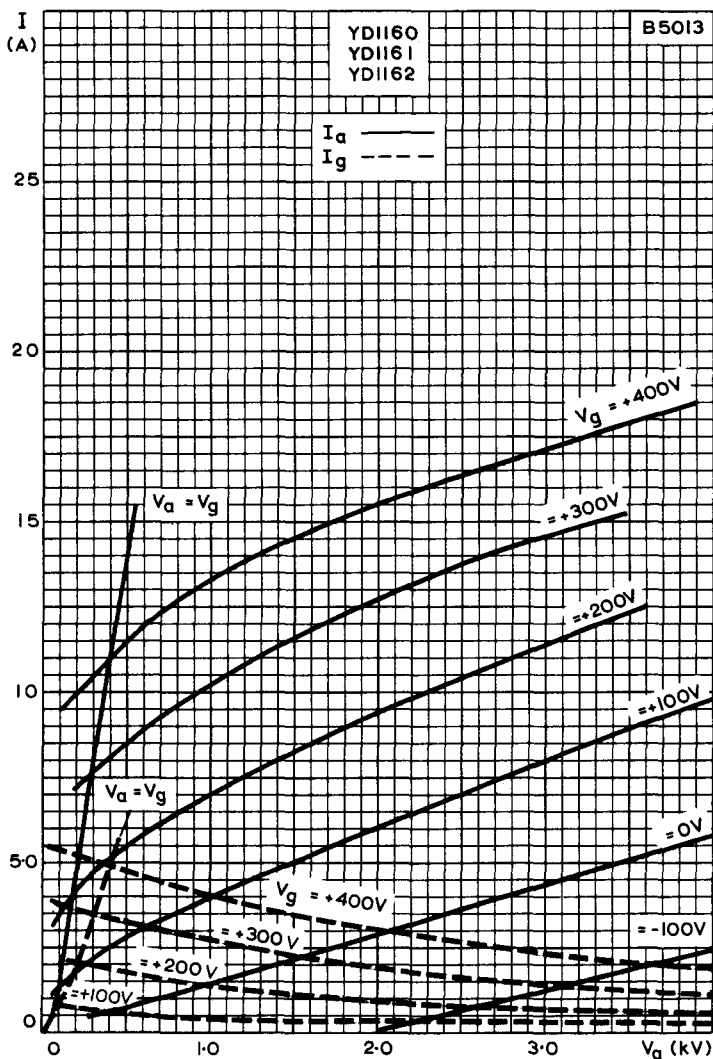
ANODE AND GRID CURRENTS PLOTTED AGAINST ANODE VOLTAGE WITH GRID VOLTAGE AS PARAMETER
