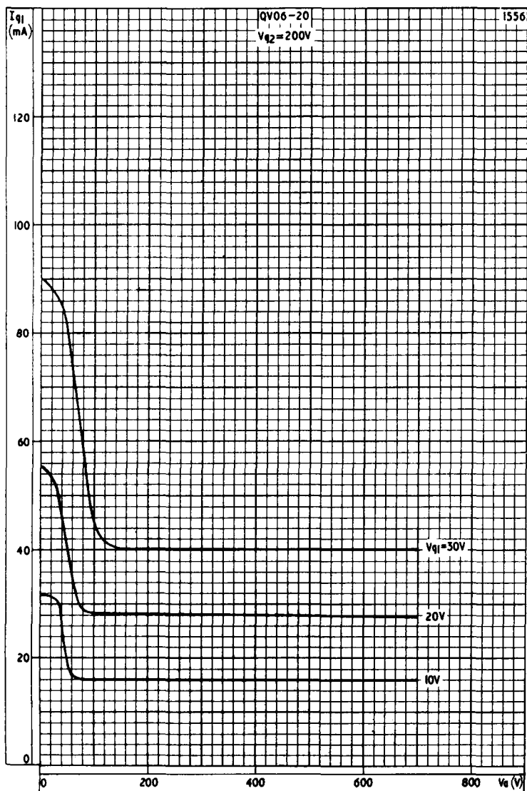
CONTROL-GRID CURRENT PLOTTED AGAINST ANODE VOLTAGE FOR SCREEN-GRID VOLTAGE=200V
