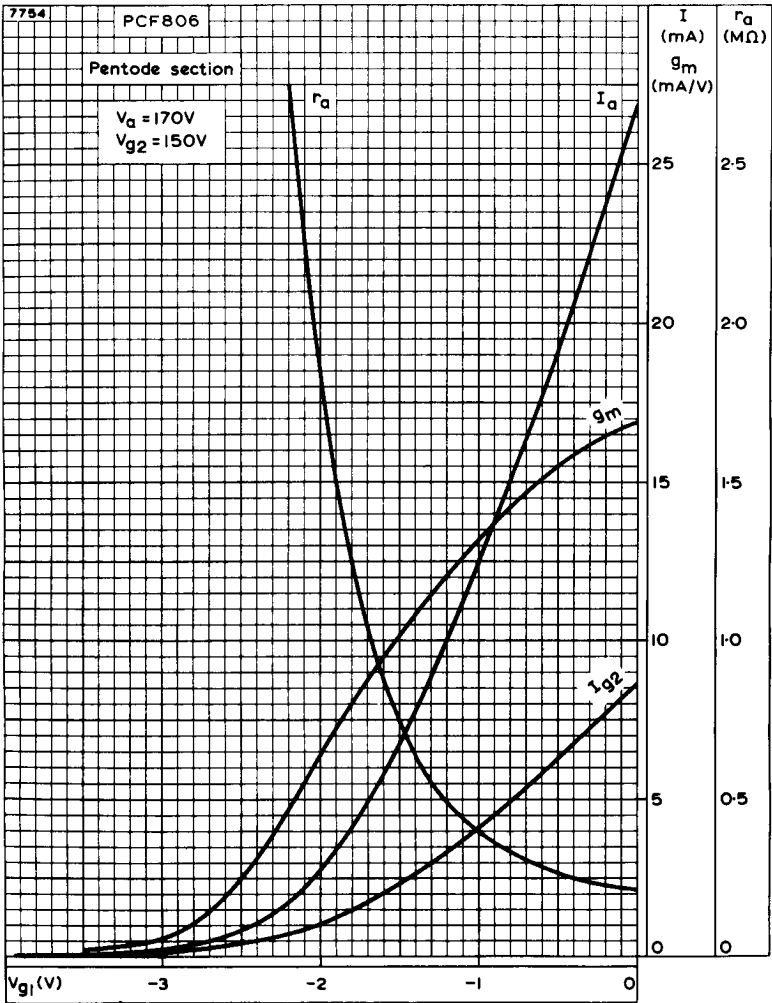
ANODE AND SCREEN-GRID CURRENTS, MUTUAL CONDUCTANCE AND ANODE IMPEDANCE PLOTTED AGAINST CONTROL-GRID VOLTAGE. PENTODE SECTION
