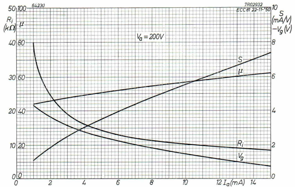
Fig. 11. Mutual conductance, amplification factor, internal resistance and grid voltage plotted against anode current, for anode voltage of 200 V.
