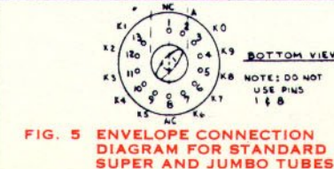
FIG. 5 ENVELOPE CONNECTION DIAGRAM FOR STANDARD SUPER AND JUMBO TUBES
