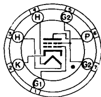
BOTTOM VIEW MINIATURE BUTTON 7 PIN BASE
