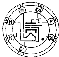
BOTTOM VIEW MINIATURE BUTTON 7 PIN BASE
