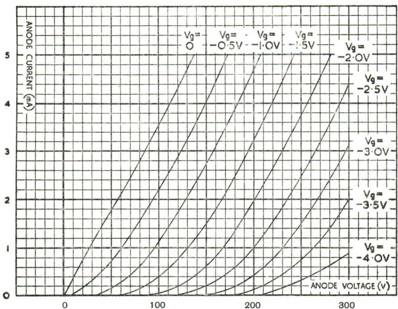
CHARACTERISTIC CURVES: g_m/V_g — Triode Section
