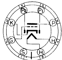
BOTTOM VIEW SMALL WAFER 8-PIN OCTAL METAL SLEEVE
